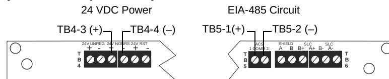
Figure D.1 AFP-100 Main Circuit Board (Top edge)
